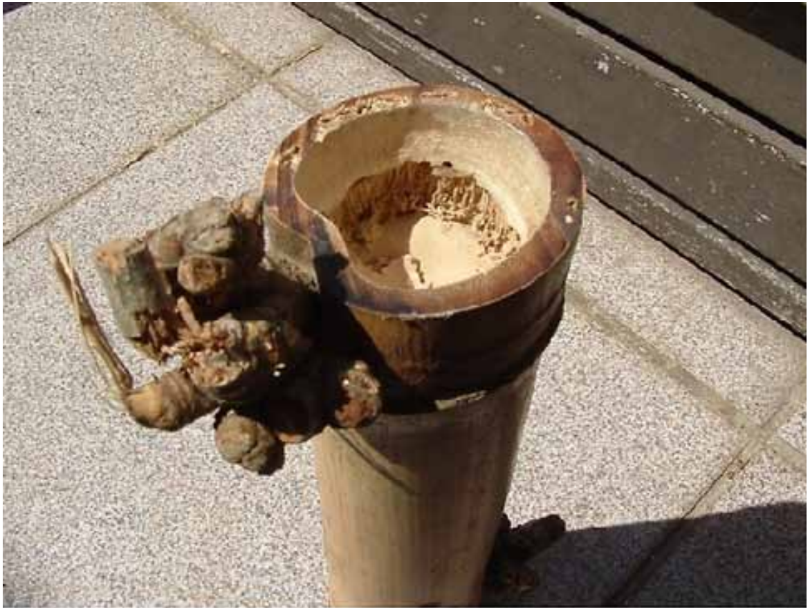
photo of cross section of a thin-walled bamboo eaten by beetles
