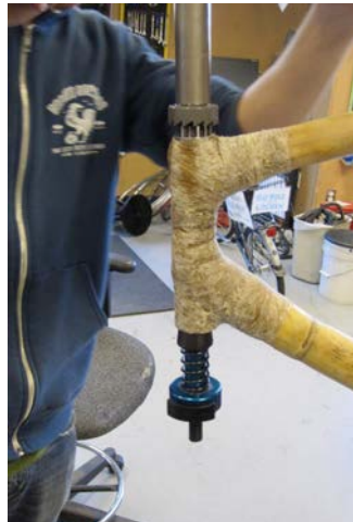
Figure 40. Simultaneously reaming and facing the head tube to accommodate a standard headset.
