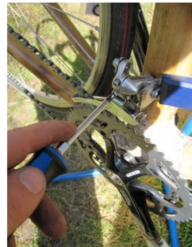
Figure 37. Adjusting the derailleur hanger while to ensure that shifting can occur on the front chain rings.
