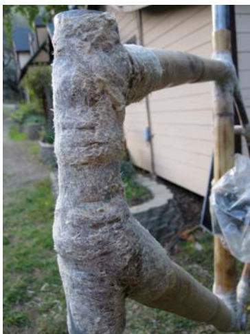
Figure 32. Head tube junction after 3 or 4 wrappings. The epoxy had not completely saturated the hemp fiber, leaving a lot of dry material in the joint that had to be sanded out and re-done.
