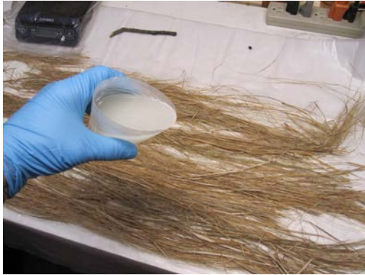
Figure 14. Pre-mixed epoxy resin is poured over the hemp fiber.
