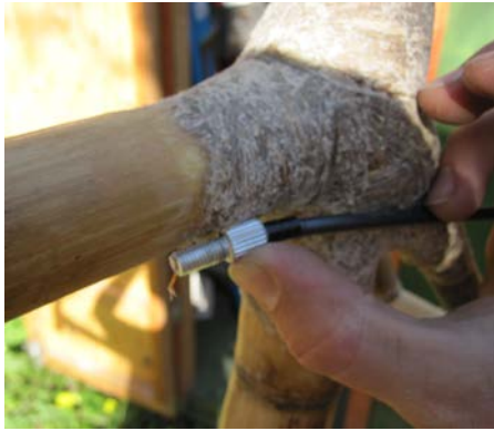
Figure 38. Positioning barrel adjusters to be glued to the frame for cable routing.
