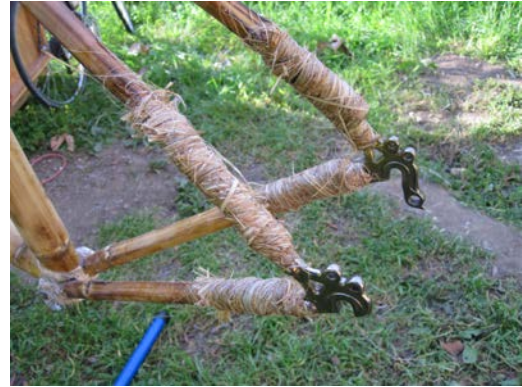
Figure 29. First wrapping of dropout connections, before sanding.
