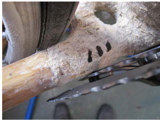
Figure 27. Lower cross brace, after some material removed to accommodate for the rear tire clearance. Material was also removed from the right side of this joint to give clearing for the small chainring.
