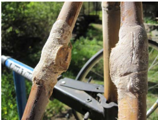
Figure 26. Removal (or amputation) of cross brace.
