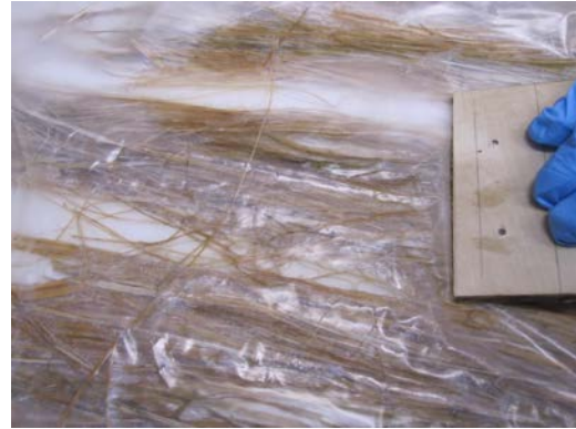
Figure 15. A wooden squeegee is used to push the resin through the fibers, ensuring they are fully saturated.
