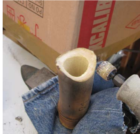
Figure 10. Using a Dremel rotary tool with a sanding attachment to bring miter to final shape.
