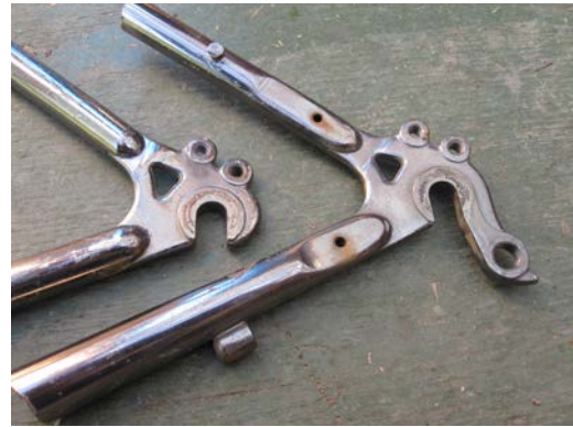
Figure 6. Rear dropouts from the same chromoly frame.
