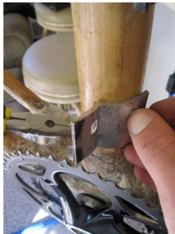
Figure 36. Shaping the front derailleur hanger to fit on the seat tube.
