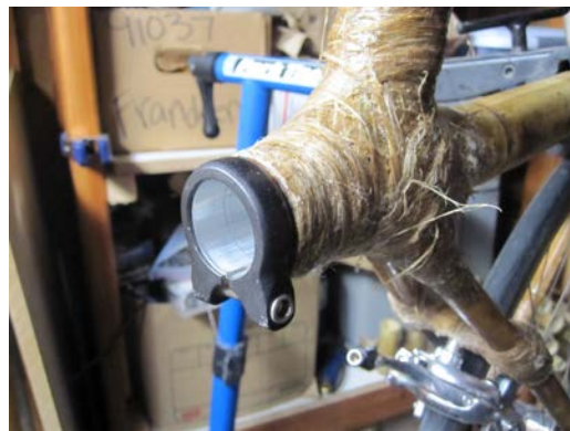
Figure 35. Seat post shim and clamp installed in bamboo frame.
