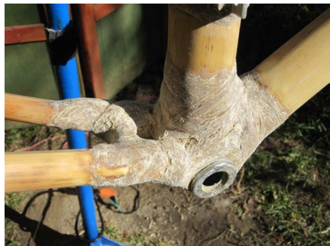
Figure 33. Final wrapping of bottom-bracket junction, after sanding. The geometry here made this quite challenging to sand and wrap correctly.
