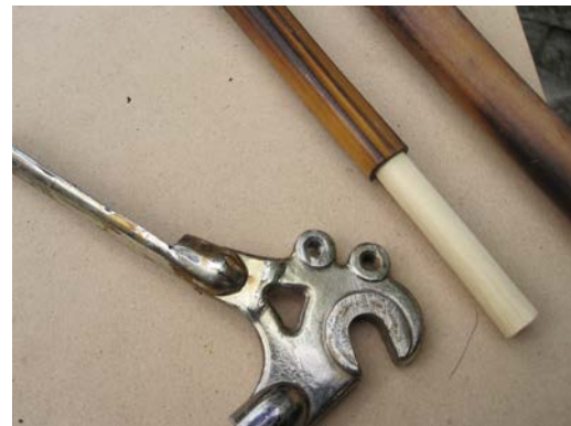
Figure 21. Rear dropout to seat stay assembly shows halved chromoly tubing, bamboo stay, and solid bamboo plug.
