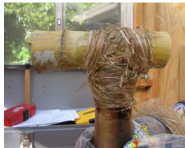
Figure 12. Hemp fiber wrapped around a joint and saturated with epoxy resin.
