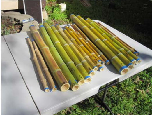
Figure 7. Bamboo poles prior to heat treatment, cut to approximate length. Extra poles were cut to ensure there would be enough usable material for one bicycle.
