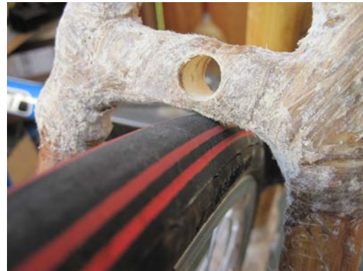
Figure 25. First iteration of upper cross brace was too close to the rear tire.
