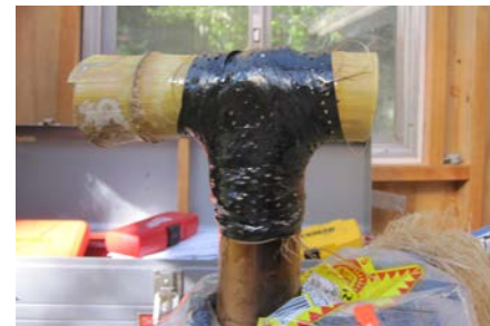
Figure 13. Perforated electrical tape is wrapped around joint to apply pressure, and to squeeze out excess epoxy resin.
