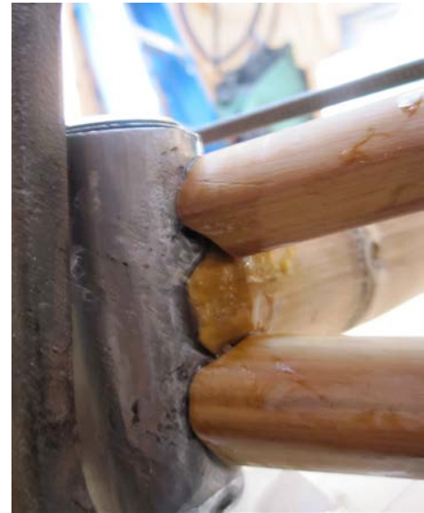
Figure 23. Junction between rear stays and bottom bracket shell shows poor contact in miter joints.
