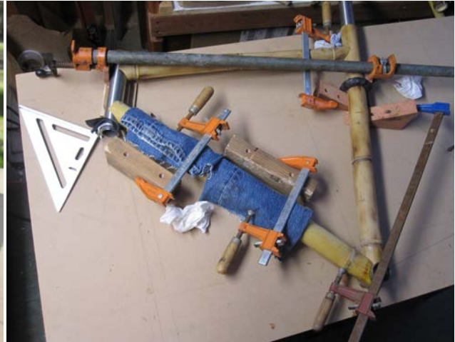
Figure 19. The front triangle as it was glued and clamped together.
