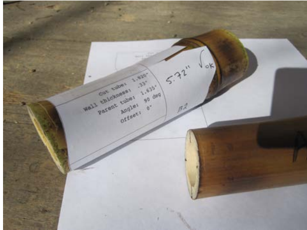
Figure 9. Tube mitering software used to transfer mitering profile onto Bamboo.
