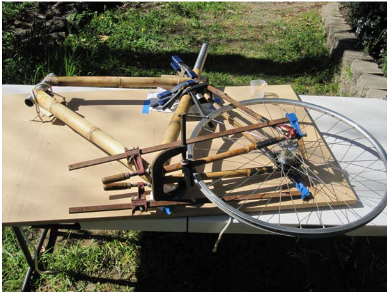
Figure 22. Using the back wheel in the MDF jig to correctly align and attach the rear stays.
