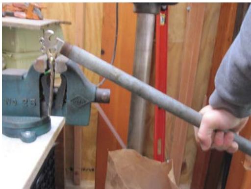
Figure 20. Using a lever arm and a vice to bend dropouts to the correct angle.
