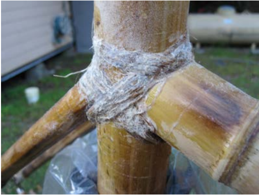
Figure 28. First wrapping of upper seat-tube junction, after sanding.
