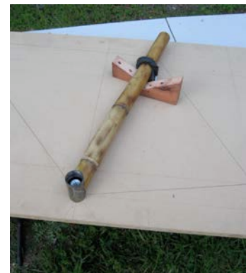
Figure 17. Bottom bracket and set tube held securely to MDF jig.
