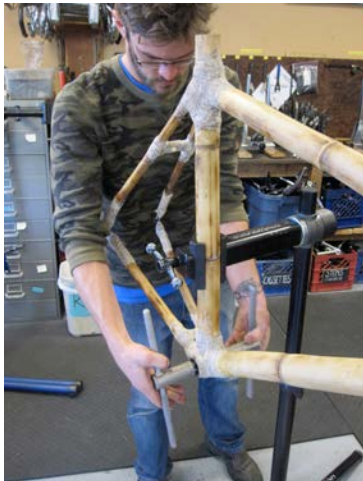
Figure 39. Chasing the threads of the bottom bracket shell.
