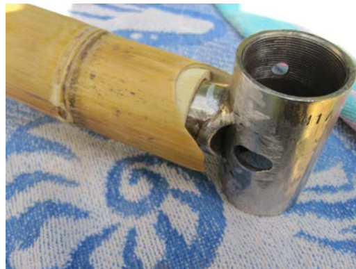
Figure 16. Bottom bracket shell to seat tube assembly, showing miter and sleeve to ensure a tight fit.
