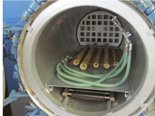
Figure 8. Bamboo poles in autoclave prior to final heat treatment.
