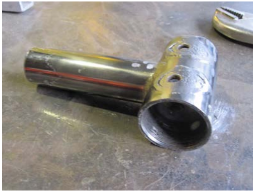
Figure 5. Bottom bracket shell after removal from a chromoly mountain bike frame.
