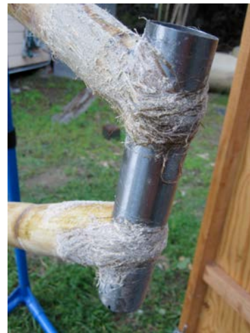
Figure 31. Second wrapping of head tube junctions, with fibers positioned to give tensile strength in the directions of the tubing.
