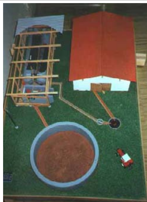
Figure 24: A model of an agricultural digester in Germany with two horizontal steel tanks, a gas storage bag and a co-generation unit in a container.
