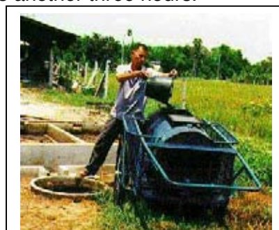
Figure 42: Drying of digested sludge and sludge disposal in Thailand
