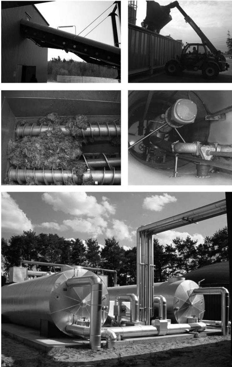
Figure 3.8 Equipment for upstream processing Closed belt conveyor (above left), Feeding the bioreactor (above right) Feeder (vielfraß®) for agricultural plant (middle left), Pump chute (middle right), Hygienization installation (below).
