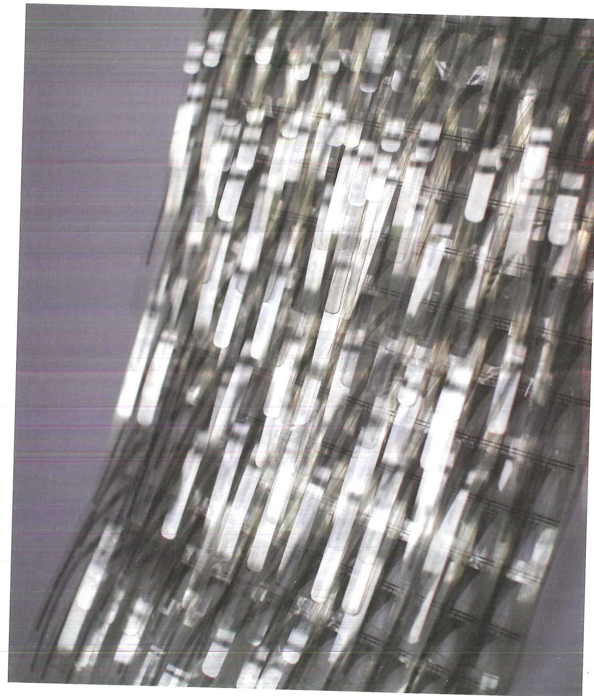
Moya, a flexible low-cost building material developed by Charlotte Slingsby, is composed of thin sheets of polyvinylidene fluoride reinforced with bendable, plastic-encased filaments that react to pressure – such as wind – to generate a charge and harvest energy.
