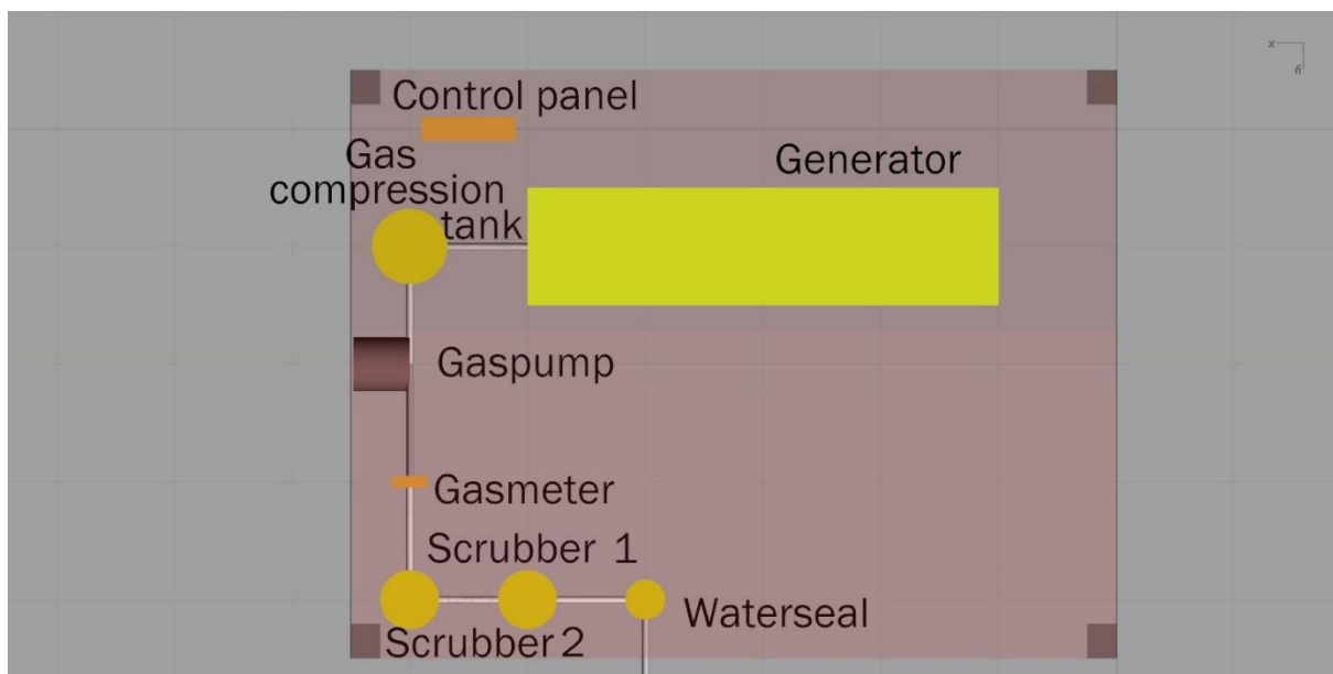
FIGURE 9 TOP VIEW GAS TREATMENT & GENERATOR HOUSING
